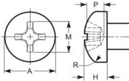
This type of recess has a large center opening, tapered wings, and blunt bottom, with all edges relieved or rounded.
